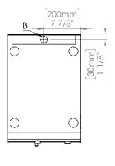
NOTES: A- WATER DRAIN, 1.2" O.D. B- ELECTRIC CONNETOR, 220V 1PH 60Hz
